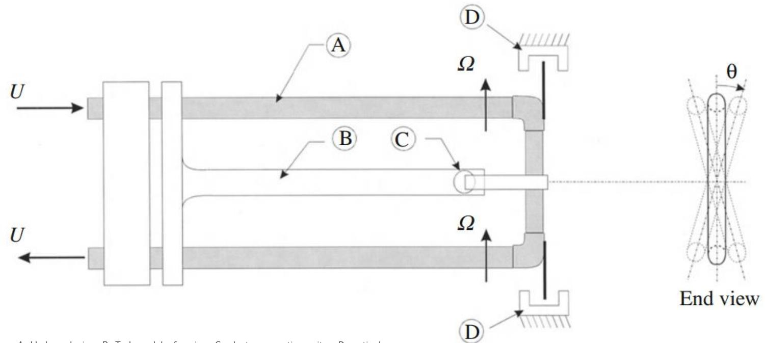
A: U-shaped pipe; B: T-shaped leaf spring; C: electromagnetic exciter; D: optical sensors
