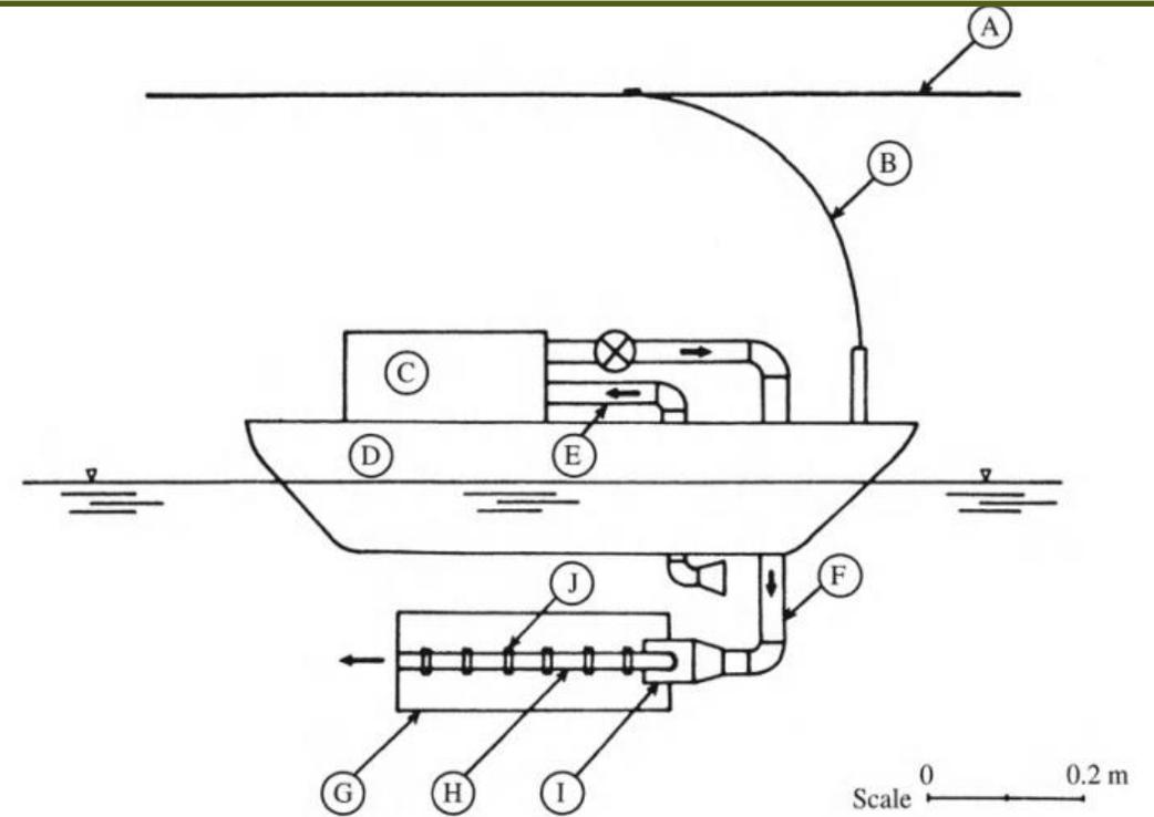
or; B: 'trolley-type' conductor; C: motor-pump unit; D: catamaran;
