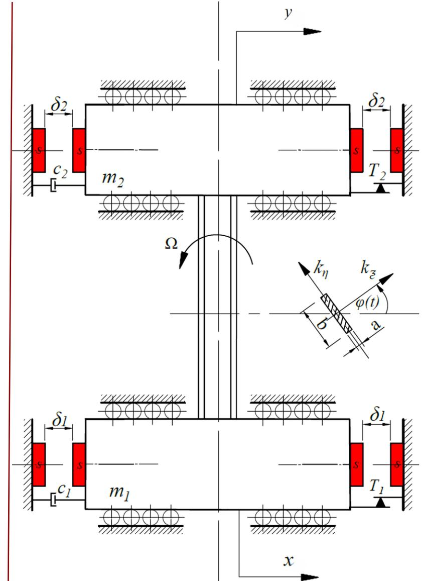
Fig. 8. 2DOF mechanical parametric oscillator
