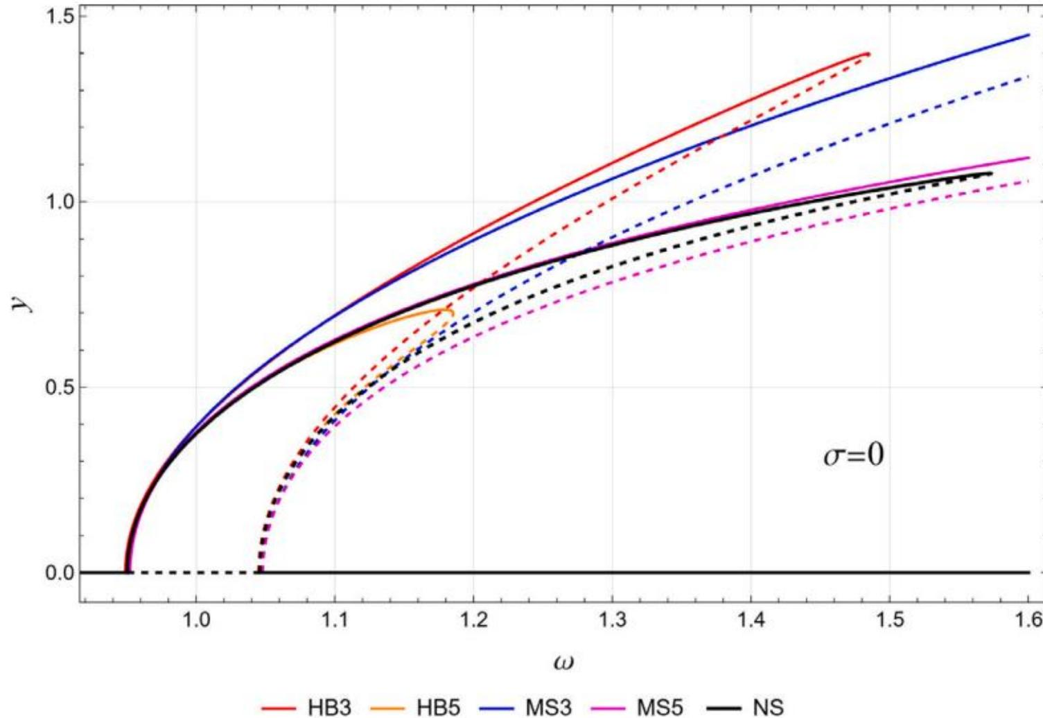
Fig.5: Branches of trivial solutions and periodic orbits (amplitudes), for  $\sigma = 0$ , obtained using different analytical approaches: harmonic balance method for stiffness characteristics described by a 3rd (HB3) and 5th-degree polynomial (HB5), multiple scale method for stiffness characteristics described by a 3rd (MS3) and 5th-degree polynomial (MS5), compared to the numerical solution.
