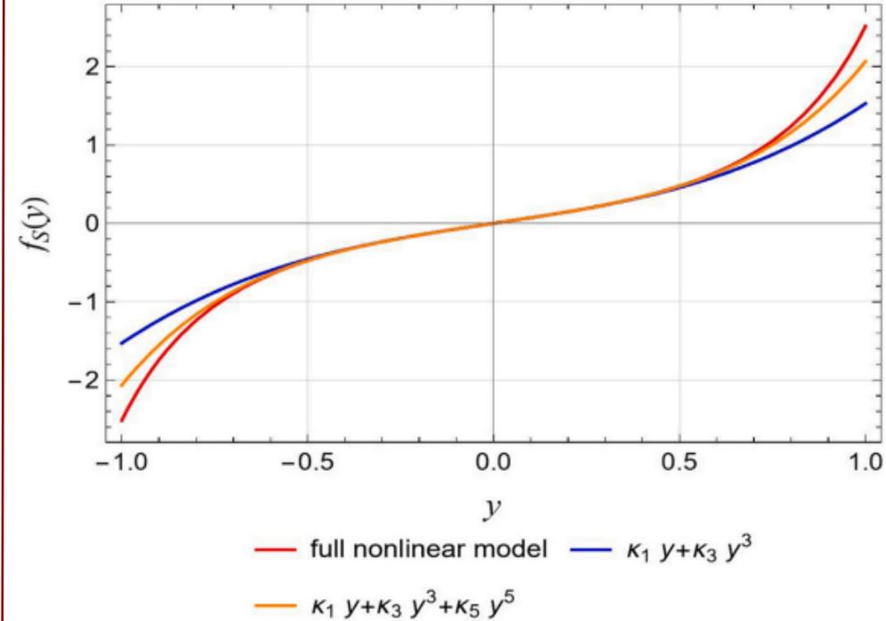
**Fig. 2.** Stiffness characteristics for full nonlinear model and its approximation by a 3rd and 5th degree polynomial
