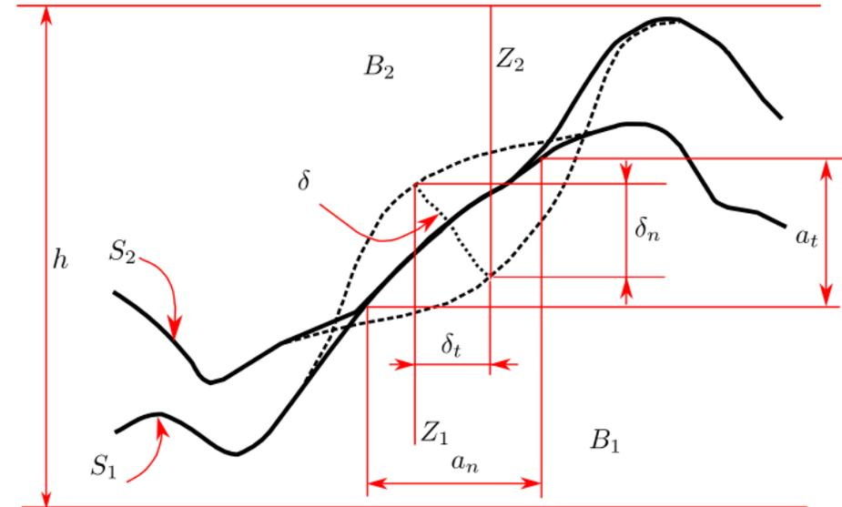
Fig. 2 Cross-section of a typical asperity contact showing projections of deformation and contact areas. Solid lines represent deformed surfaces; dotted lines indicate undeformed surfaces [2].
