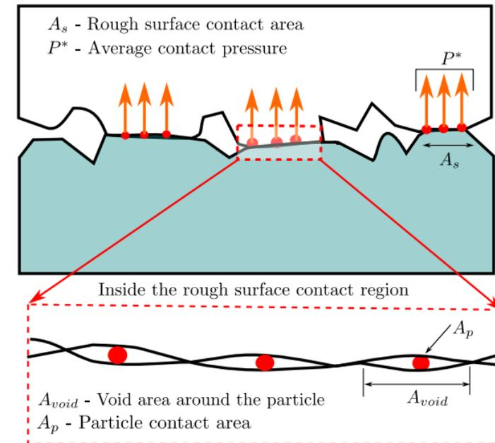
Fig. 3 Illustration of a stacked rough surface and statistical model [3].
