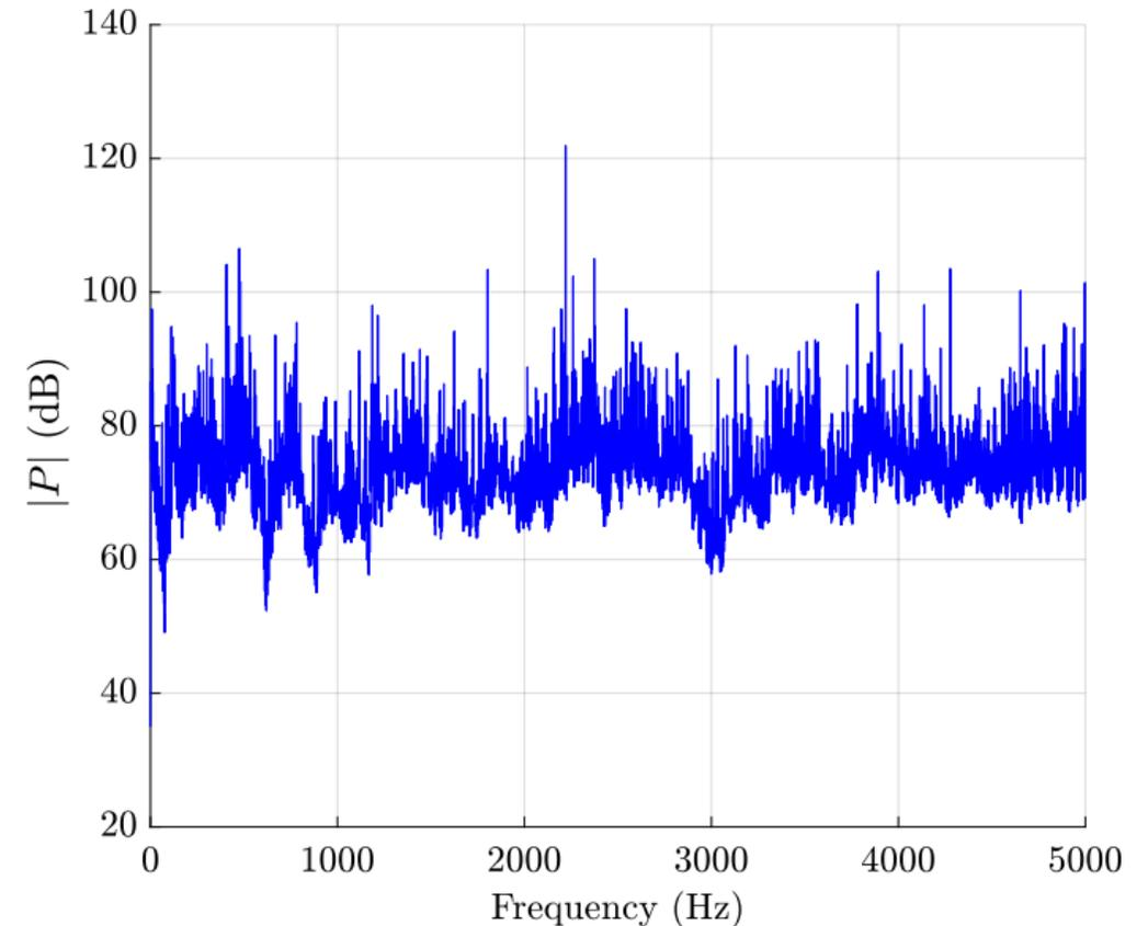
Fig. 12 Power spectrum of the microphone signal capturing rough friction in a 2-DOF mechatronic system consisting of a beam and a table driven by a PMLSM.
