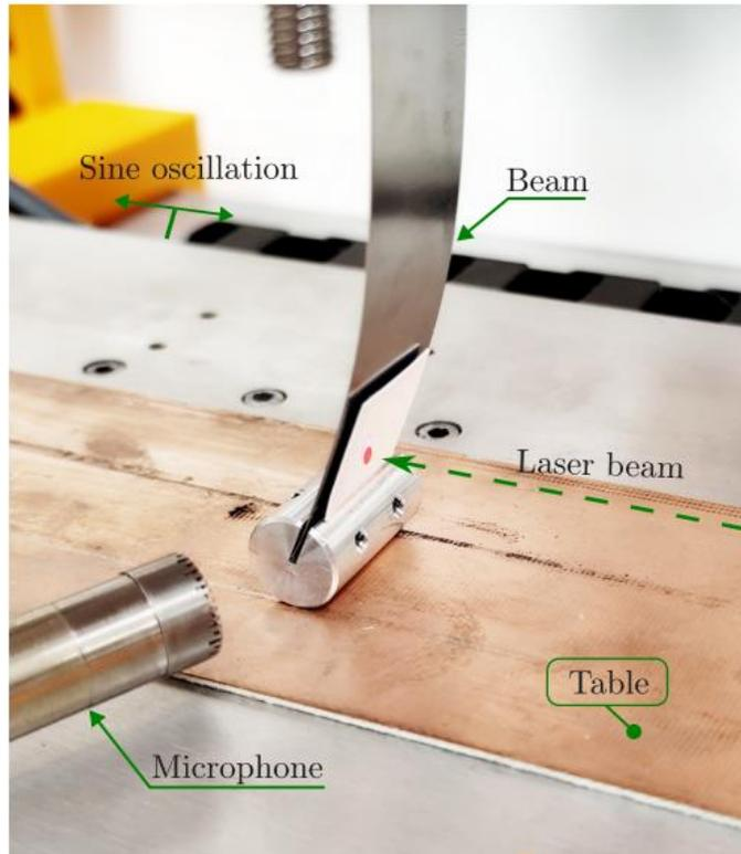
Fig. 9 The laboratory experiment with acoustic wave emission in friction-induced stick-slip vibrations in a 2-DOF mechatronic system consisting of a beam and table surface
