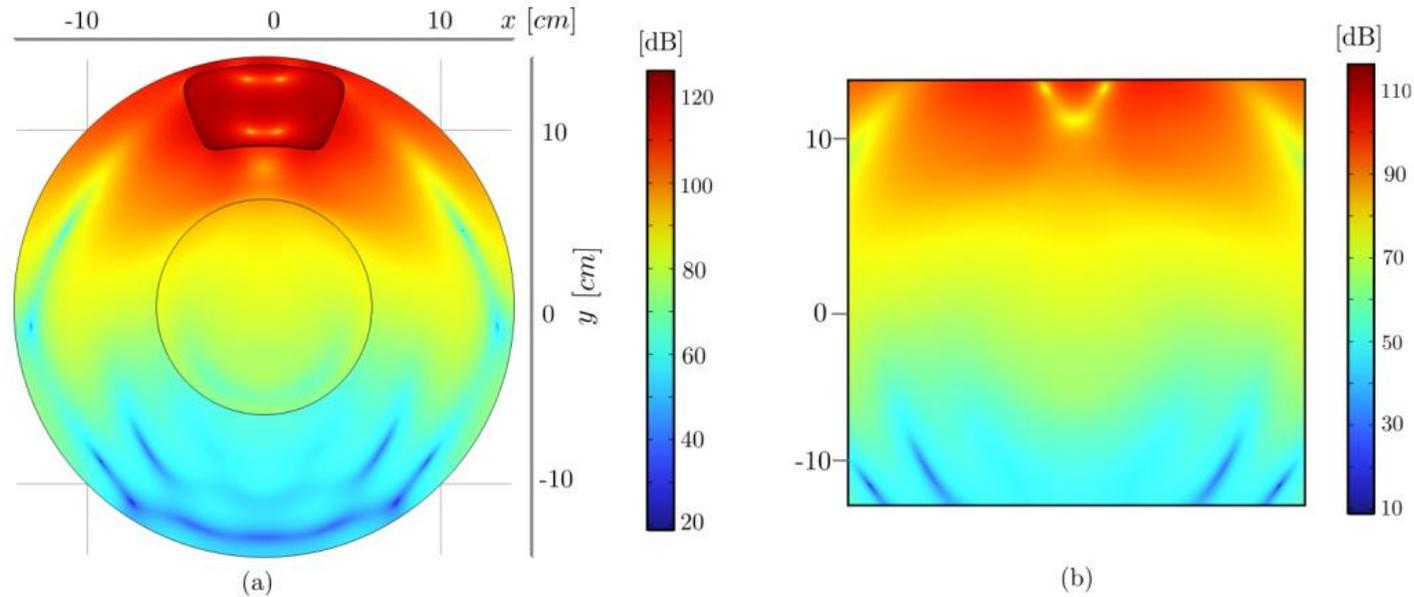
Fig. 7 Acoustic intensity estimated in COMSOL during stationary regime for  $\mu = 0.72$  at a frequency of 6426 Hz. (a) Disc and pad (BEM); (b) near field
