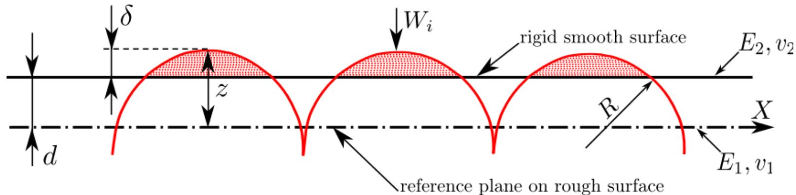
Fig. 1 Schematic of contact of a regular patterned rough surface against a smooth plane surface [1]
