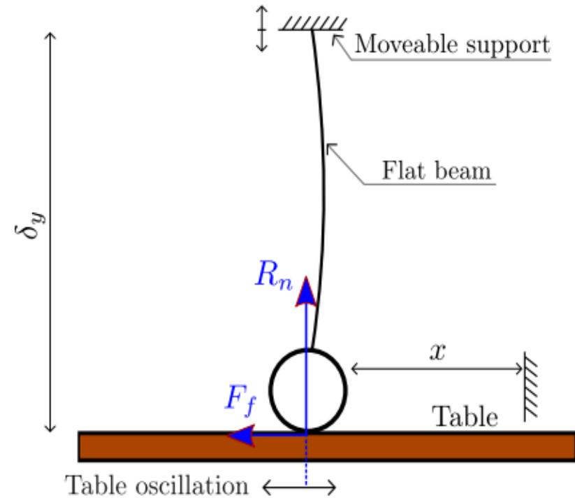
Fig. 10 Physical model of the table and the flexible flat beam dynamical interaction in a frictional contact ( $R_n$  – the normal reaction force,  $F_f$  – the surface frictional force).
