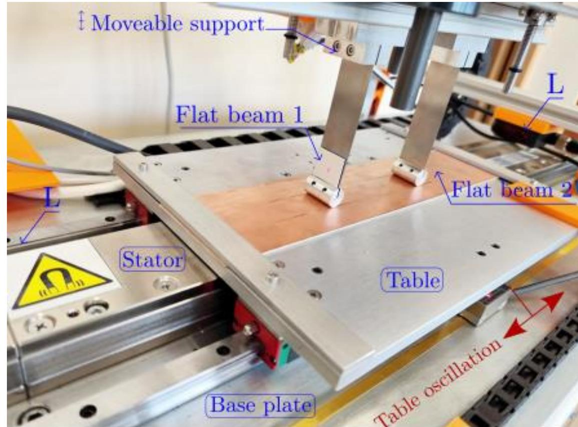
Fig. 8 Experimental station [Olejnik et al.,2025]
