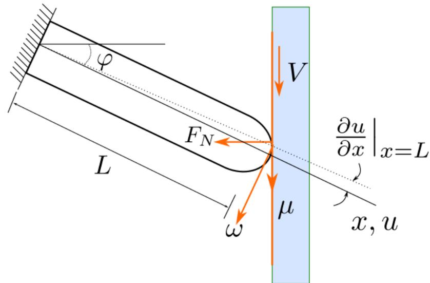
Fig. 4 Schematic figure of the rod and the disk [4]
