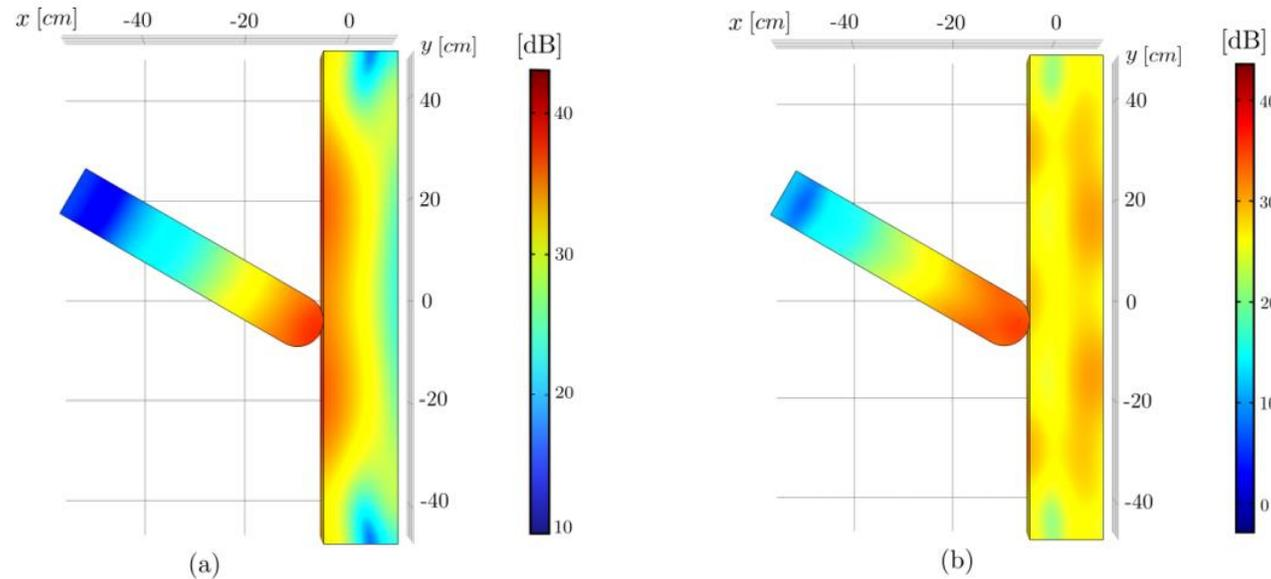
Fig. 5 Sound Pressure Level distribution estimated in COMSOL on the beam and disc surfaces at: (a) 750 Hz, (b) 1250 Hz
