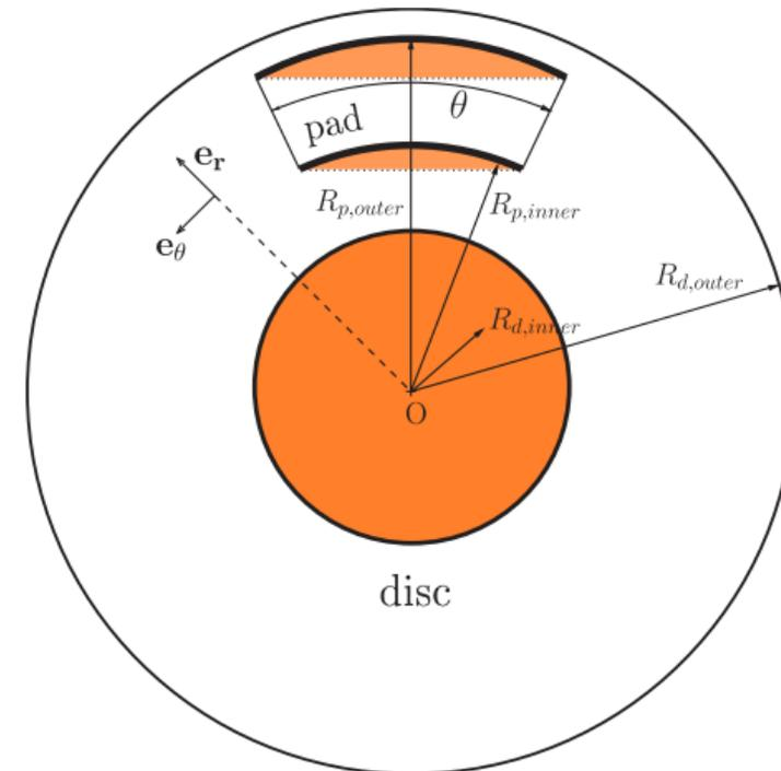
Fig. 6 Illustration of the geometrical parameters [7]
