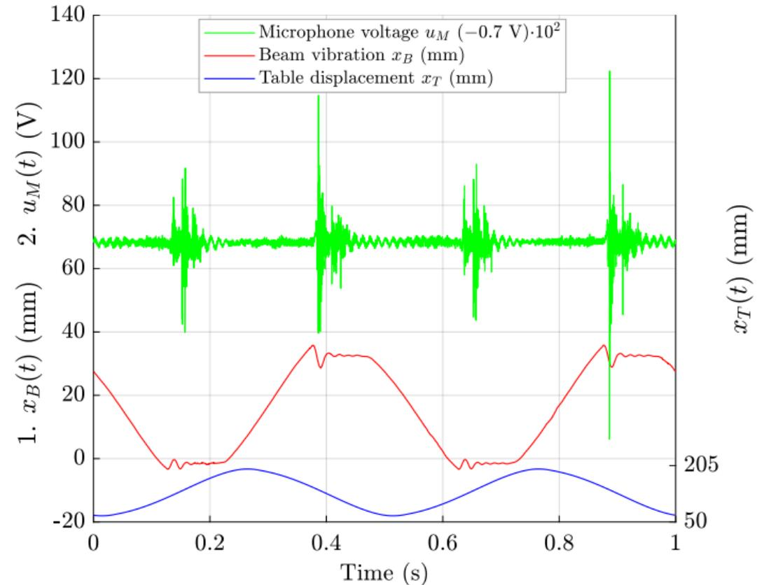
Fig. 11 The real friction-induced vibration profile with coexisting acoustic (rough) friction in a 2-DOF mechatronic system consisting of a beam and a table surface.
